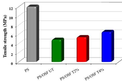
**Figure 3: Effect of treatment concentration on the tensile strength of composites PS/OSF**
