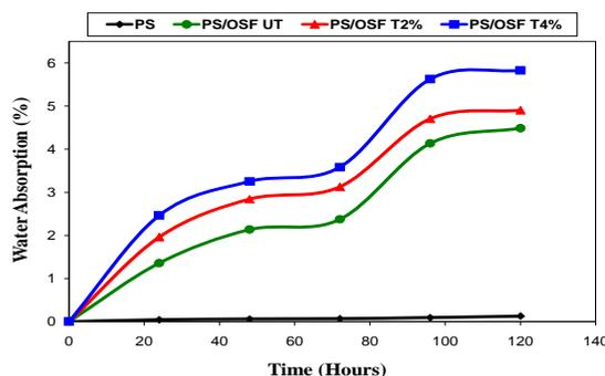
Figure 6: Effect of treatment concentration on water absorption of composites PS/OSF
