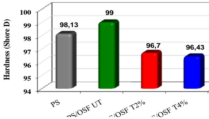
Figure 5: Effect of treatment concentration on the hardness of composites PS/OSF
