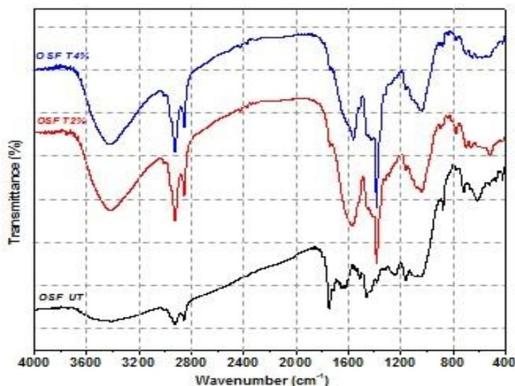
Figure 1: FTIR spectra of untreated (OSF UT), Alkali treated for different concentration of treatment (OSF T2%, OSF T4%).
