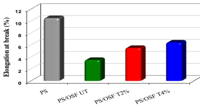
**Figure 4: Effect of treatment concentration on the elongation at break of composites PS/OSF**
